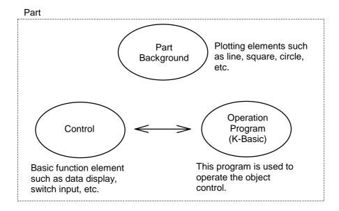
The table below shows the types and functions prepared for each control. For details of each command, refer to the K-Basic program description manual.
